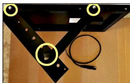
Using (2) #10-16 x 3/4" screws, secure the larger bottom brackets to front corner of solar panel on each side using pre-drilled far corner holes. Using same screws secure the smaller brackets to one of the three provided predrilled holes on the solar panel. Finish by using knob bolt and wing nut with washers to connect the two brackets in one of the adjustment holes provided on the bottom bracket. Each circle in the image represents the connections being made on each side of the solar panel.
