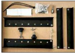
Your installation package should include (6) #10 - 16 x 3/4" and (6) #10 - 16 x 2.5" self-drilling screws, matching nut driver, (2) 5/16" knob bolts with wing nuts, 4" of sealing tape, 2 zip ties and the mounting brackets.
