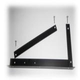
**2**. Locate the  $6 - \frac{3}{4}$ ". Notice the adjustable 9" leg holes are offset. Attach the 9" leg to the bottom mount with the offset closest to the inside of the angle. (Depending on your roof pitch, this may have to be moved for best adjustment later)
